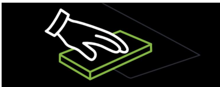
When a surface is contaminated or corroded you have to sand the surface first and clean with Isopropylalcohol and a Lint-free cloth
