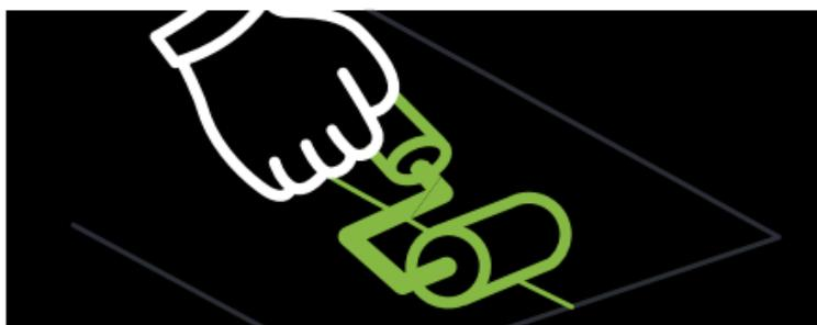
Finally connect the substrates and press them well with a pressure roller for better adhesion. Review and test the connection of the substrate before using it for the intended application.
