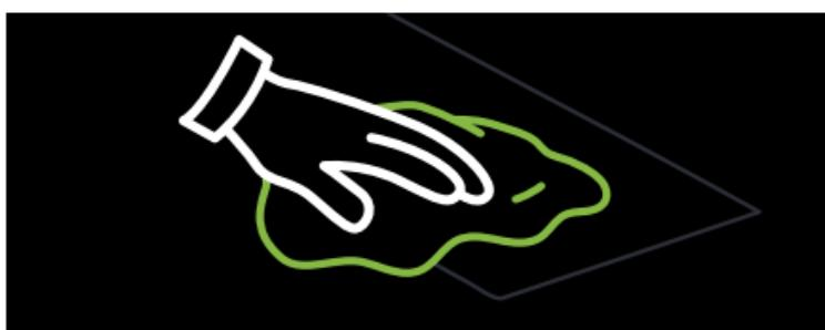
Substrates have to be dry. Clean always in one direction and in one movement.
